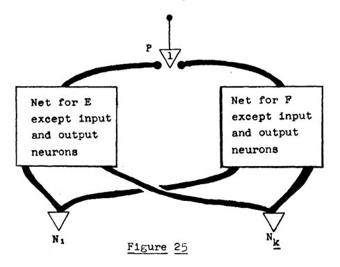
The heavy bundle of neurons leading to P from the left are those which would be required in the net for E separately; like-wise from the right in the net for F. The bundle from  $N_1$  toward the left, those from  $N_1$  in the net for E, to the right in the net for F, etc. The fact that the output neurons for the two given nets had no axons leading back in insures that they still operate independently of each other in this combination.
