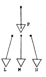
$\underline{P}(\underline{t}) \equiv \underline{L}(\underline{t}-1) \vee \underline{M}(\underline{t}-1) \vee \underline{N}(\underline{t}-1)$   $\underline{F1g}. 2$
