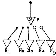
$\begin{bmatrix} (\underline{N}_1 \& \underline{N}_2) \lor (\underline{N}_1 \& \underline{N}_3) \lor (\underline{N}_2 \& \underline{N}_3) \end{bmatrix} \& \underline{N}_4 \& \underline{N}_5 \\ \begin{bmatrix} \underline{N}_1 \lor \underline{N}_2 \end{pmatrix} \& (\underline{N}_1 \lor \underline{N}_3) \& (\underline{N}_2 \lor \underline{N}_3) \end{bmatrix} \lor \underline{N}_4 \lor \underline{N}_5$
