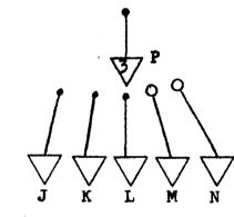
$\underline{P}(\underline{t}) \equiv \underline{J}(\underline{t}-1) \& \underline{K}(\underline{t}-1) \& \underline{L}(\underline{t}-1) \& \underline{M}(\underline{t}-1) \& \underline{M}(\underline{t}-1) \\ \underline{Fig}. \ \underline{1}$
